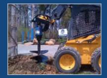
The heavy duty series augers are an economical option that is still a quality planetary drive. This unit comes in 3 models to cover most flow ratings in the skid steer and tractor market. The durable housing, the hex shaft, and the 4 year warranty make it a reliable attachment to own.
