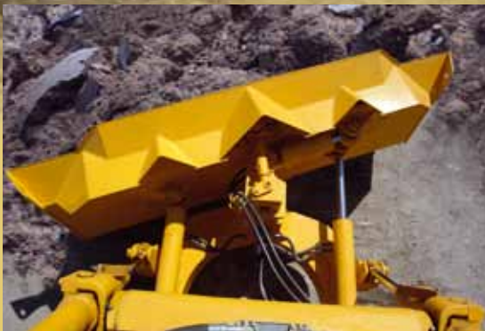
6-way hydraulic angle blades of 5 cu.yd (3.8 cu.m) used with wide track (WT) and 5.2 cu.yd (4.0 cu.m) used with low ground pressure track (LGP) are applicable for versatile operations such as finish grading, spreading material and light land clearing.
