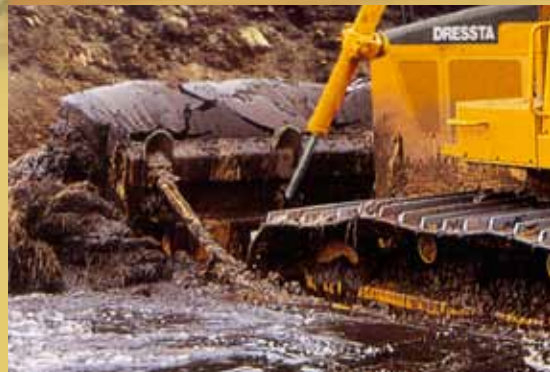
Straight blade of 4.7 cu.yd (3.6 cu.m) used with 85 in (2.16 m) gauge and 37 in (940 mm) track shoes (LGP) is designed for soft, swampy areas. This blade is equipped with hydraulic tilt cylinder to perform efficiently landscaping operations.
