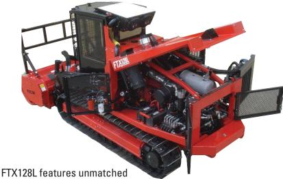
service and accessibility for daily service checks and cleaning as well as opening up for periodic scheduled maintenance. All service checks can be made from standing on the ground with an easy reach.
