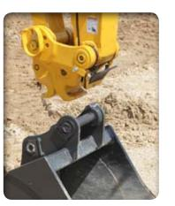
**POWER-A-TACH**<sup>®</sup> allows hydraulic attachment changes with the flip of a switch. The operator leaves the seat only to engage and disengage the safety pin.
