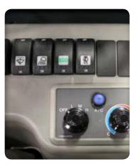
**TRUE EFFICIENCY** ECO mode and auto deceleration improve fuel economy, decrease noise and lower emissions by reducing engine speed when not necessary.
