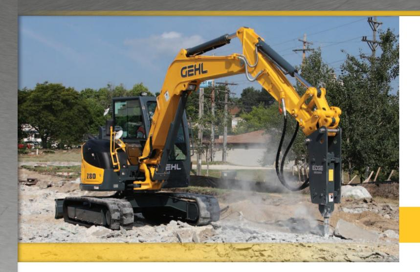
The Gehl Z80 compact excavator brings power and intelligence together in one zerotail-swing model. Power is provided with a 54.6 hp (40.7 kW) Yanmar Interim Tier IV diesel engine. Intelligence comes with the ECO mode and auto deceleration, improving fuel economy and lowering emission levels.
