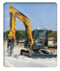
**ON-DEMAND HYDRAULICS** provide no loss of hydraulic performance during simultaneous movements, allowing smooth operation even while using the boom and arm during turning.
