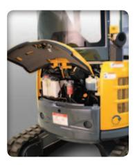
EASY SERVICE ACCESS is achieved with the large rear door, removable side covers, and removable cover beneath the operator's seat.
