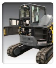
EASY SERVICE ACCESS Large, rear hood opens easily to expose the battery, engine oil, air filter and cooling system.
