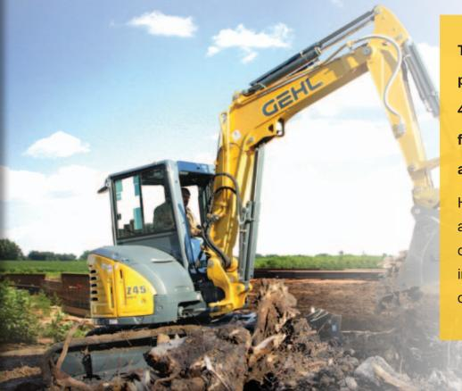
Turn to the ALL-NEW highperforming Gehl Z45 GEN:2 4.5 metric ton compact excavator for additional digging force in a zero-tail-swing configuration. High-performance hydraulics and a powerful Yanmar diesel engine combine to provide the ultimate
