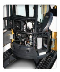
**ENHANCED SERVICE** ACCESS is achieved with two large rear doors, a swing-open side access panel, and removable covers beneath the operator's seat.
