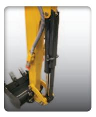
EXTRA PROTECTION on the bucket, dipper and boom cylinders is provided by plate spring cylinder guards. The upper structure's lower frame is reinforced by high-strength steel covers.
