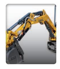
**ON-DEMAND HYDRAULICS** incorporate four hydraulic pumps which require less engine power and provide no loss of hydraulic performance during simultaneous movements.
