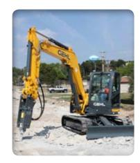
ZERO-TAIL-SWING design allows the superstructure to rotate entirely within the tracks without overhang, allowing operation close to walls and other obstacles.
