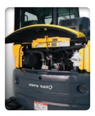
SERVICEABILITY and daily maintenance checks are made easy with the large removable side panels, flip-open rear engine door and under-seat access panel.
