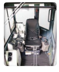
provides a spacious, ergonomic operating environment. The cab is mounted on five silicon, oil-filled vibration to the operator.
