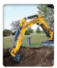
**HIGH-PERFORMANCE BOOM** is constructed with thick side plates and a single-pin mounted design for optimal strength and durability.
