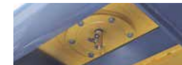
Fuel tank drain valve.
