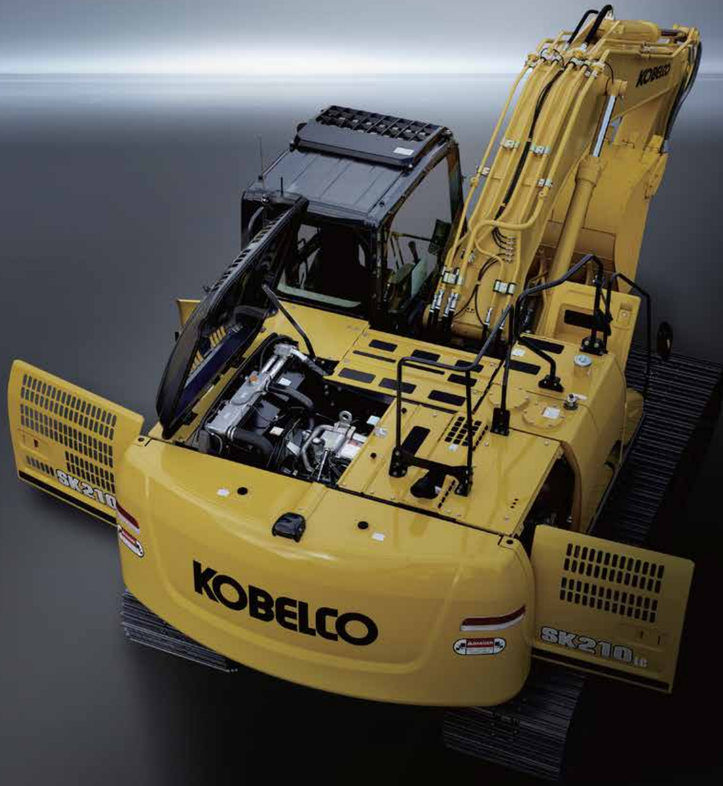
Air Cleaner (double element) Radiator Fuel Filter (with built-in water separator) Engine Oil Filter
