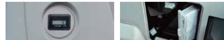
Hour meter can be checked while standing on the ground. Air conditioner filter can be easily removed without tools for cleaning. One for outside air and one for inside air.
