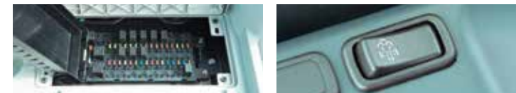
Easy-access fuse box. DPF Manual Regeneration Switch
