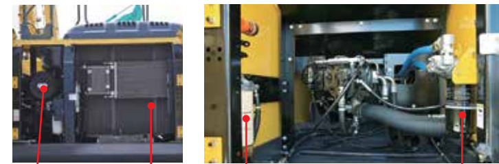
Air Cleaner (double element) Radiator Fuel Filter (with built-in water separator) Engine Oil Filter
