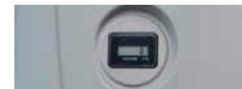
Hour meter can be checked while standing on the ground.
