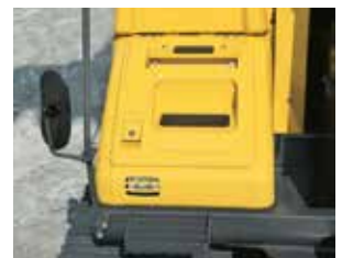
Front mounted three steps instead of only two for easy safe access.
