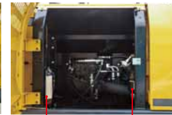
Fuel Filter (with built-in water separator)
