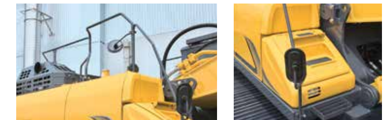
Handrails Front mounted three steps instead of only two for easy safe access.
