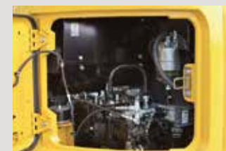
● Protective panel separates the pump compartment from the engine
