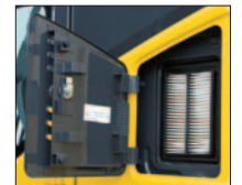
External air conditioner filter
