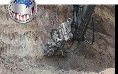
Recommended Excavator/Carrier Size Class: 35 - 50 tons
