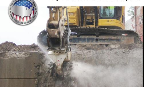
Recommended Excavator/Carrier Size Class: 25-45 tons
