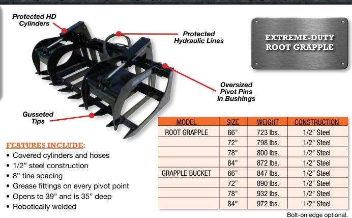
The extreme duty root grapple has proven itself for many years as an effective and reliable land clearing attachment. The front cross tube helps float the grapple while surface raking, and keeps it from diving too deep while root raking. The well engineered geometry of this grapple and the high quality cylinders give it the best clamping force in the industry. All pivot points are 1-1/4" pins in greasable bushings. This grapple is ready to tackle the toughest of jobs!
