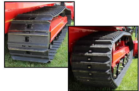
Strong Traction from Steel Tracks with Single or Triple Grousers or Metal Imbedded Rubber Tracks for Pavement Applications
