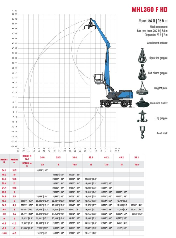
Capacity values are stated in pounds I metric tons. The pump pressure is 5,221 psi I 360 bar. The values, in accordance with ISO 10567, represent 75% of the static tipping load or 87% of the hydraulic lifting force (marked \*). Values apply to 4-pt supported slewing operations over 360 degrees on a firm and level surface.
