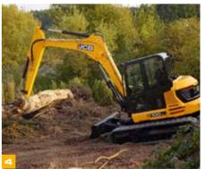
Excellent SAE service rating equates to greater uptime for both the JCB 90z and 100c. Our machines are more serviceable courtesy of features like a gas-strutted 30-degree tilting cab. You don't need special tools to operate this either, so routine checks are quicker to perform than ever.
