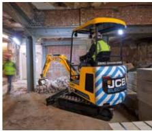
Auto-idle reduces the engine speed (RPM) when the machine is idle for a set amount of time, to preserve battery charge.
