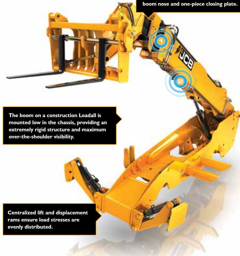
The boom on a construction Loadall is mounted low in the chassis, providing an extremely rigid structure and maximum over-the-shoulder visibility.
