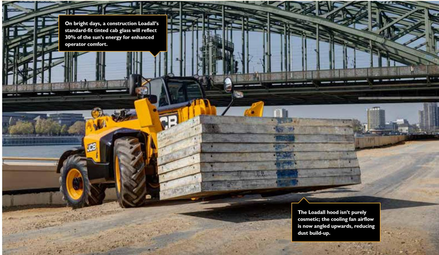
On bright days, a construction Loadall's standard-fit tinted cab glass will reflect 30% of the sun's energy for enhanced operator comfort.
