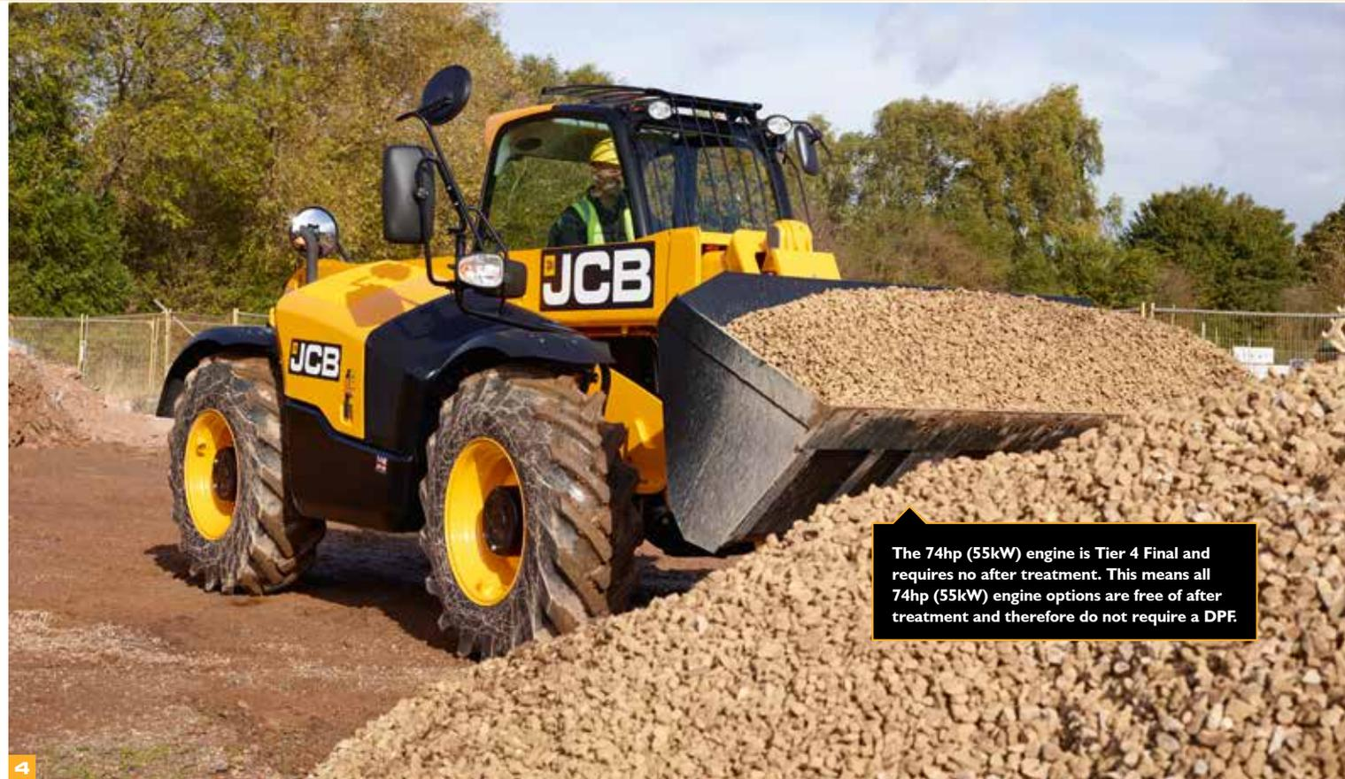
The 74hp (55kW) engine is Tier 4 Final and requires no after treatment. This means all 74hp (55kW) engine options are free of after treatment and therefore do not require a DPF.
