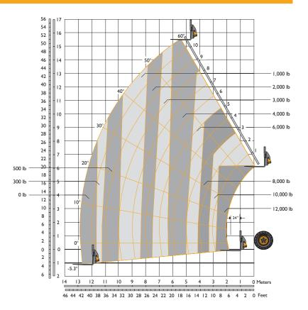
These load charts are for the rated capacity of the machine with 72" wide standard carriage and 48" pallet forks. Complies with ANSI/ITSDF B56.6 Automatic rear axle stabilization (RAS) system.
