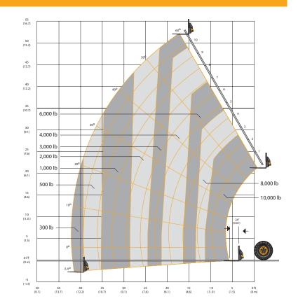
These load charts are for the rated capacity of the machine with 66" wide standard carriage and 48" pallet forks. Use only JCB approved attachments and check the relevant load chart for the machine model. Complies with ANSI/ITSDF B56.6 Automatic rear axle stabilization (RAS) system.
