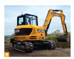
The heavy duty boom cylinder guard provides excellent protection with optional arm and crowd cylinder guards available for more arduous applications.
