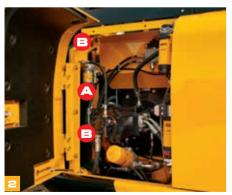
(A) Hydraulics oil filters (B) Fuel filters
