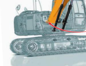
By using graphite impregnated bronze bushes, we've reduced the JSI3I's boom and dipper greasing intervals to 1000 hours for normal applications.
