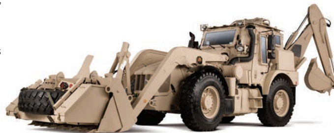
Built in Savannah, the fully armored JCB High Mobility Engineer Excavator (HMEE) is the world's toughest backhoe. The JCB HMEE is currently deployed by the U.S. Army in Iraq and Afghanistan.
