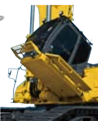
Tilting cab to reduce fatigue during demolition in high places (optional)
