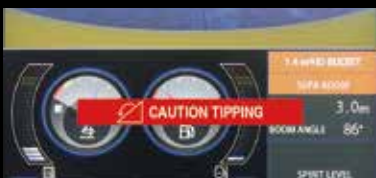
Stability warning display
