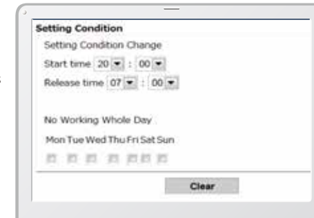
Engine start alarm outside prescribed work time
