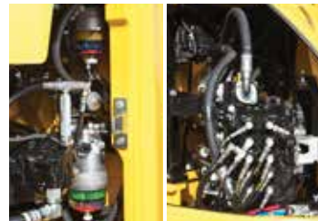
Fuel water separator/Fuel filter/Control valve
