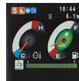
DEF tank level gauge
