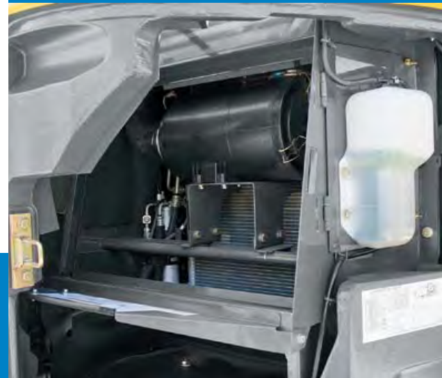
2-Stage engine air filter and radiator systems are accessible after removal of pre-filter screen.
