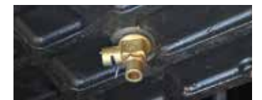
Fuel tank features bottom flange and large drain valve for easy maintenance.
