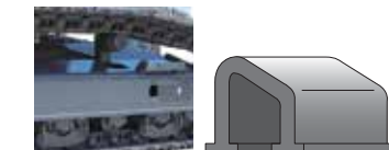
Special sloped crawler side frame design is easily cleaned of mud.
