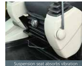
Suspension seat absorbs vibration
