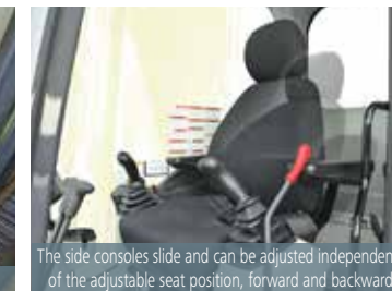
It takes 25% less effort to move the operation lever, which reduces fatigue over long working hours or continuous operations.
