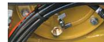
Fuel tank drain valve.
