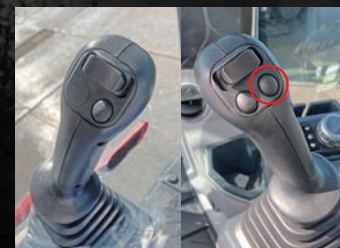
Proportional slides on the joysticks with power boost switch (right control lever)
