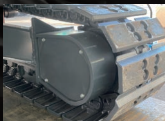
Reinforced travel motor cover
