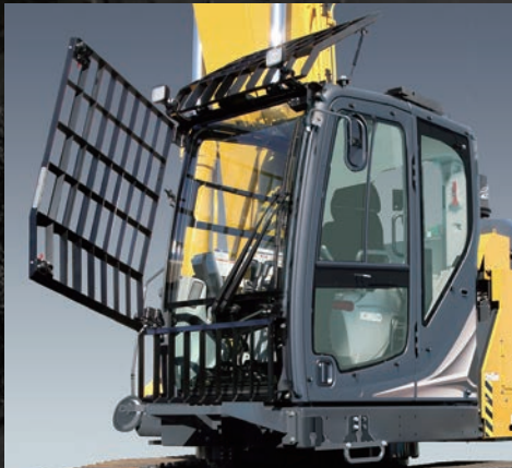
Easy to clean open/close cab guard (upper front window and skylight)
