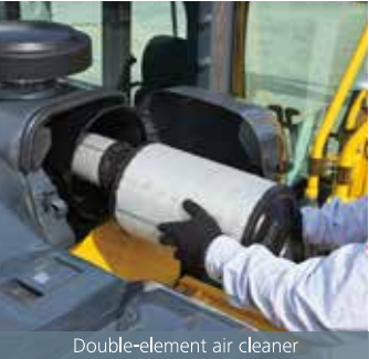
Double-element air cleaner
