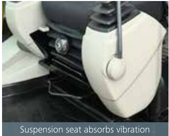
Suspension seat absorbs vibration
