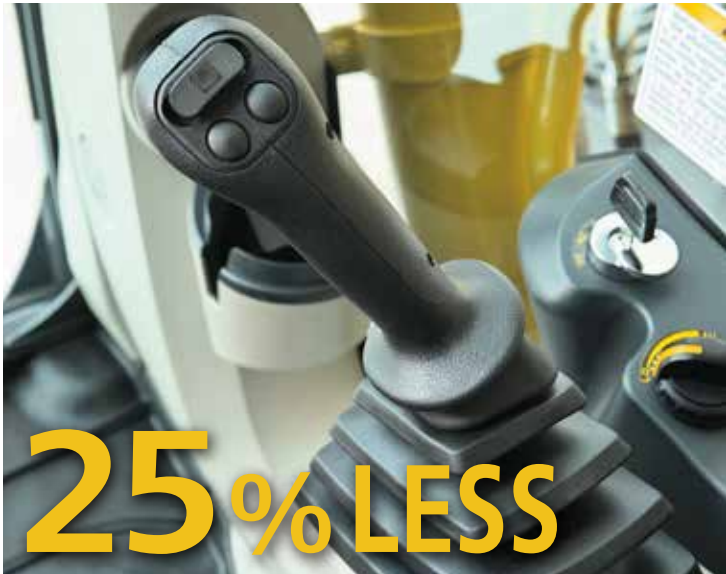
It takes 25% less effort to work the operation lever, which reduces fatigue over long working hours or continuous operations.
