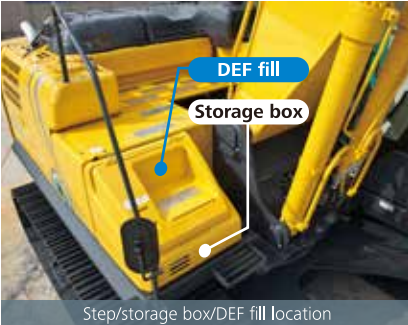
Step/storage box/DEF fill location
