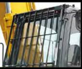
Wire Mesh or Vertical Bar Front Cab Guard (optional)
