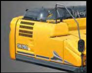
**Angled Upper Deck Guards** Angled upper deck guards run along the side of the upper body to protect door panels from impact and damage.
