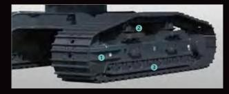
Unbeatable durability The crawlers are designed to provide unbeatable durability to take on the harshest terrain. They feature full track guides to eliminate de-tracking concerns, a reinforced guide frame built to withstand heavy impact, and large, double-support, outer flanged upper rollers unfazed by powerful vibrations.
