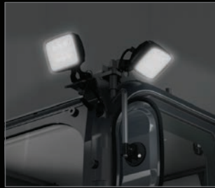
Forward and Left-Facing LED Light (Cab)
