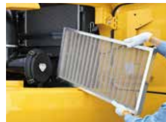
iNDr filter/radiator reservoir tank/air cleaner access.
