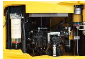
Fuel filter with built-in water-separator
