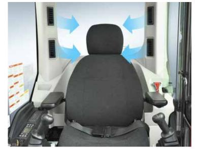
Five air outlets deliver warm or cool air directly to the operator.
