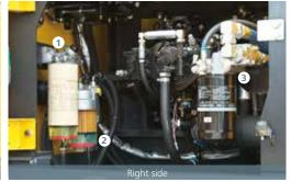
2 Fuel filter with integrated water separator
