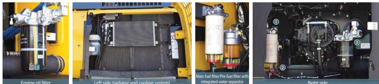
Laid out for easy access to radiator and cooling system elements
