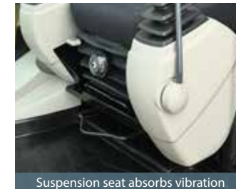
Suspension seat absorbs vibration
