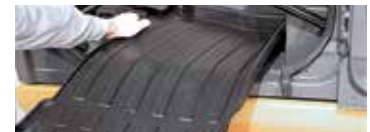
Detachable twopiece floor mat with handles for easy removal.
