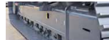
Special sloped crawler side frame design is easily cleaned of mud.
