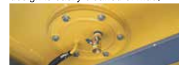
Fuel tank drain valve.
