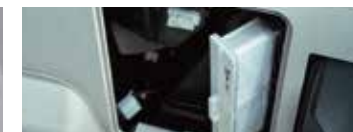
Air conditioner filter can be easily removed without filters for cleaning. One for outside air and one for inside air.
