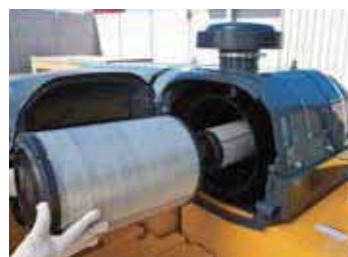
Air cleaner (double element) The double filter system provides clean and filtered air for the engine.
