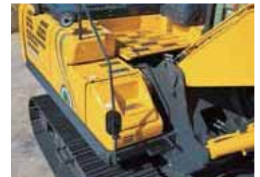
Maintenance space Large open space on top of machine to easily service and inspect engine.
