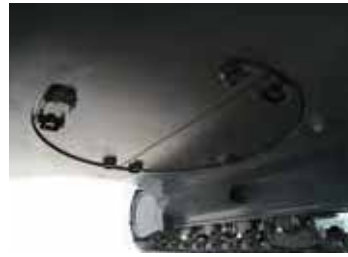
Swivel guard The lower car body structure is fitted underneath with a 0.35" (9mm) thick reinforced cover.
