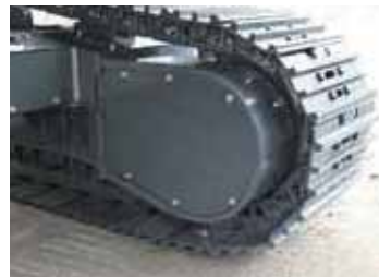
Reinforced guard for travel motor Thick steel plate used to ensure strength and protect drive motors.
