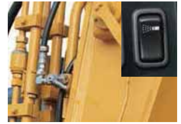
Dust suppression system (with drainage circuit) A drainage circuit is installed to drain water from the lines and prevent rust or freezing.
