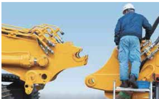
Piping connection: Hydraulic quick coupler system on the side of the boom.
