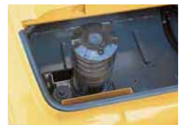
Auto lubrication system The upper body is automatically greased at specific times to reduce operator maintenance before starting work.
