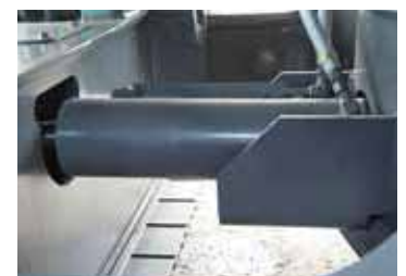
Crawler extension/retraction mechanism guard Hydraulic cylinders are protected from debris. [on SK400DLC and SK550DLC]
