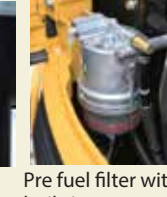
Pre fuel filter with built-in water separator
