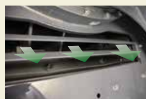
Offset duct slow down exhaust
