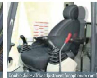
Double slides allow adjustment for optimum comfort
