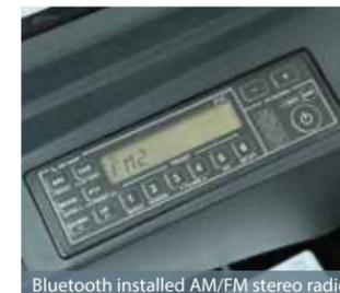
Bluetooth installed AM/FM stereo radio
