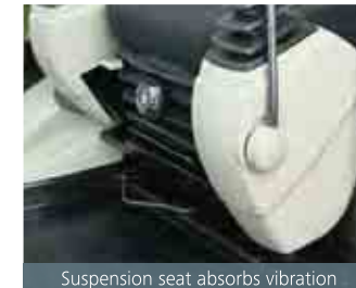
Suspension seat absorbs vibration
