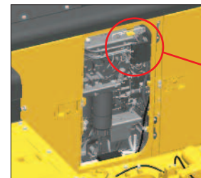
Electric priming pump switch
