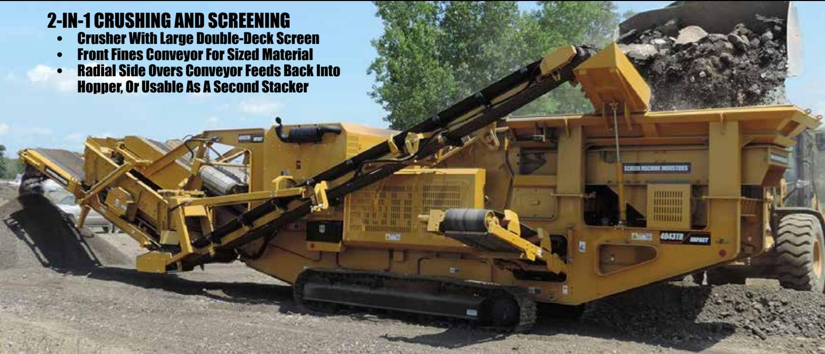
48" (1,219mm) wide fines conveyor delivers sized material off the front of the machine
