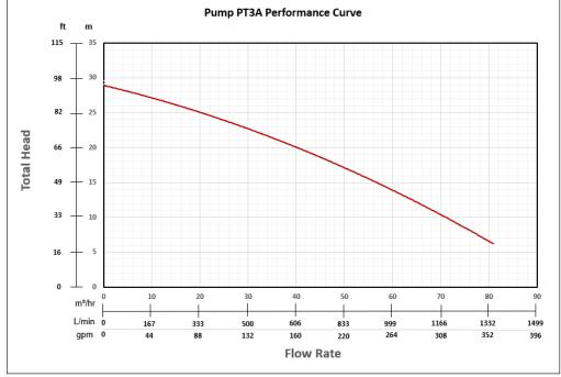
Test Standard: ISO 9906: 2012: Table 8-Pump Acceptance Grade 2B
