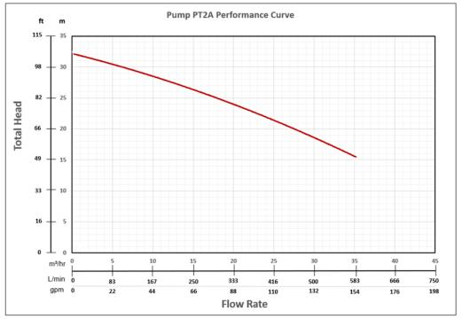
Test Standard: ISO 9906: 2012: Table 8-Pump Acceptance Grade 2B
