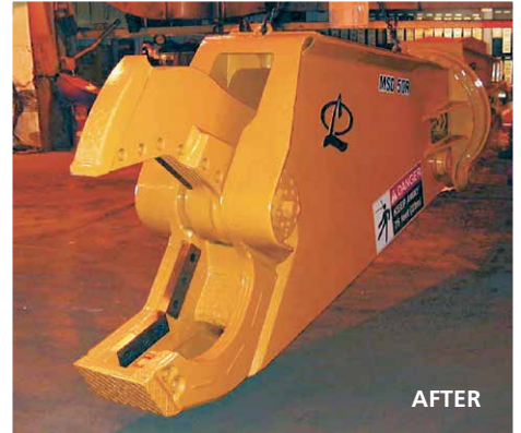
This 15 year old MSD shear, used heavily for scrap processing (above), was recently reconditioned to provide many additional years of service.
