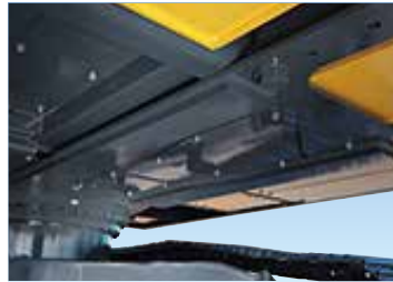
Frame is reinforced from the factory to support the heavier counterweight.
