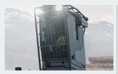
Front and roof guard for timber application
