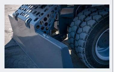
• Support blade, integrated cylinder protection
